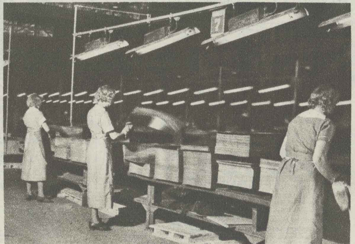
11 An operator places black plate into an automatic feeder preliminary to the process of tinning the metal. It is the thin coating of tin that keeps the steel from rusting.
