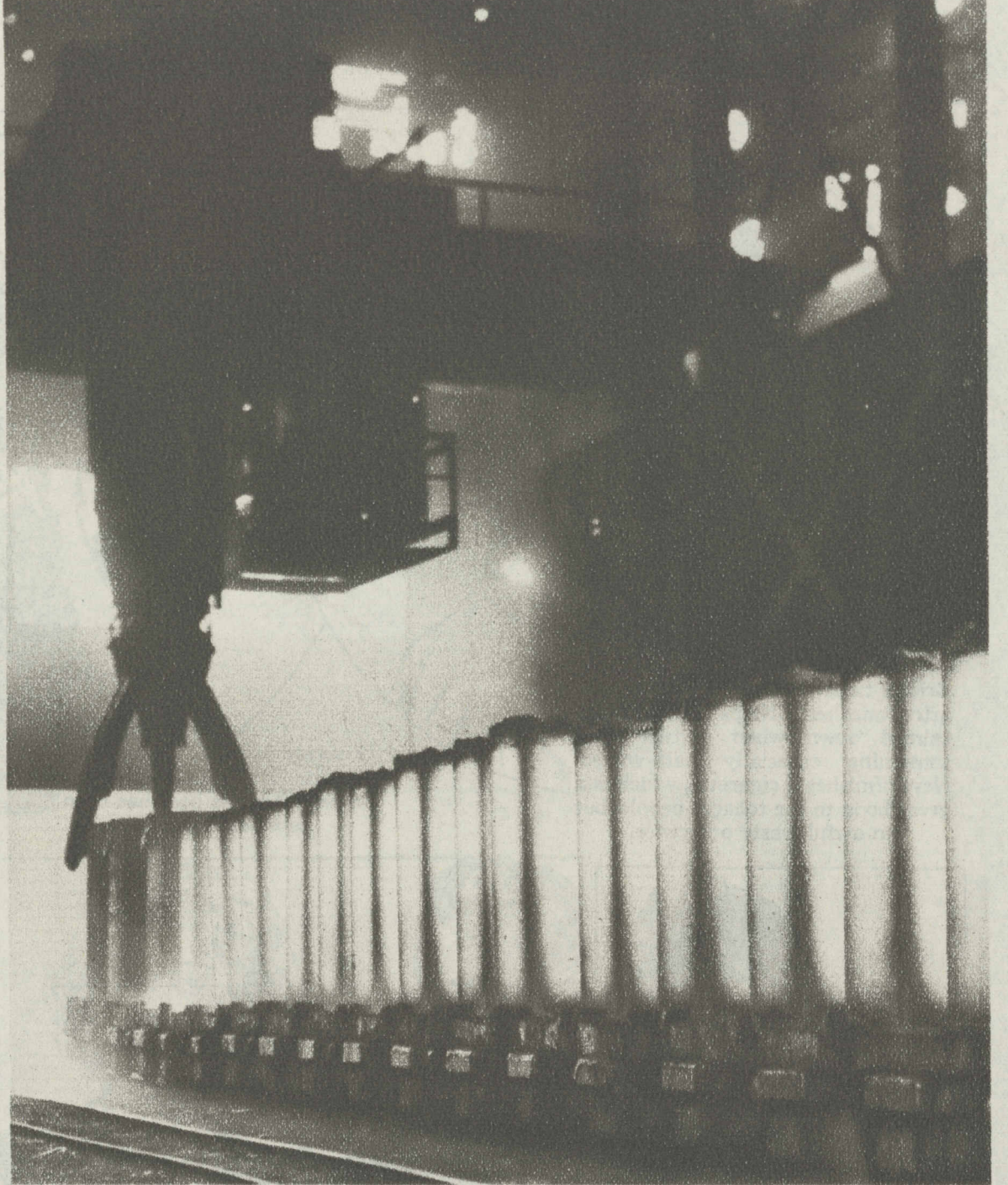
2 The ladle of molten steel from the open hearth furnace spills its fiery cargo into ingot molds, in which the metal is allowed to solidify and partially cool.
