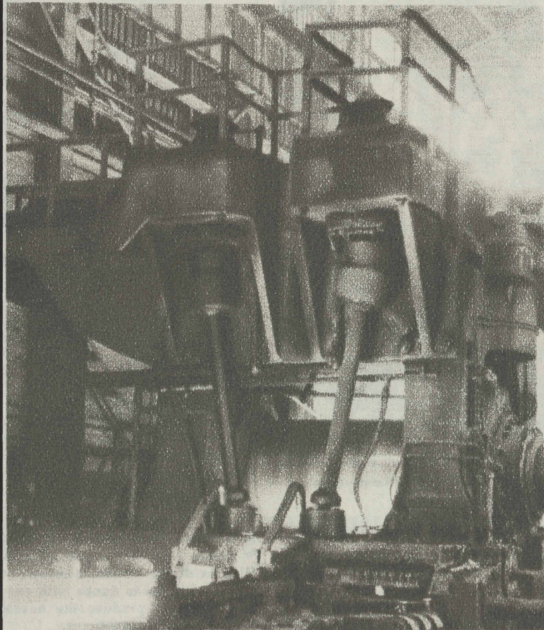
7 A roughing stand of the 78-inch continuous mill takes the steel slab after it has left the blooming mill. The slab is further reduced as to dimensions, its width being swiftly narrowed by means of vertical, or edging, rolls.
