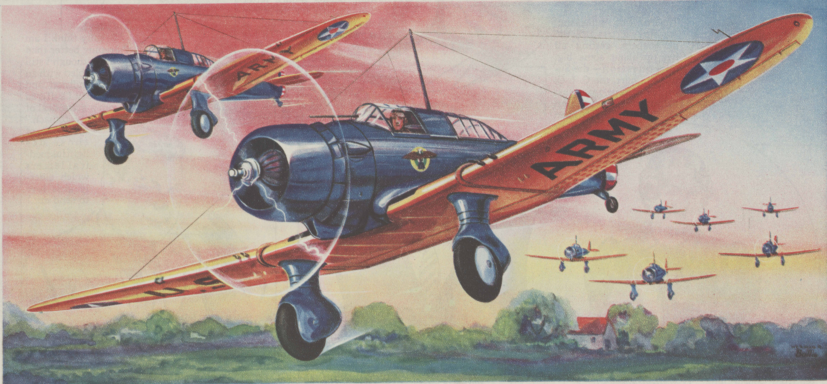
Predatory war birds: A low-flying attack squadron with Northrop A-17 airplanes. These military machines have been specially designed to attack troops, transport trains, strong points, artillery emplacements, and similar concentrated targets on the ground. Their technique is to fly as low as possible, raking their objective with machine gun fire, bombs, and gas as they swoop over it at 250 miles an hour. They arrive so suddenly and depart so swiftly after striking that there can be no reprisal. The planes each carry pilot and gunner.
