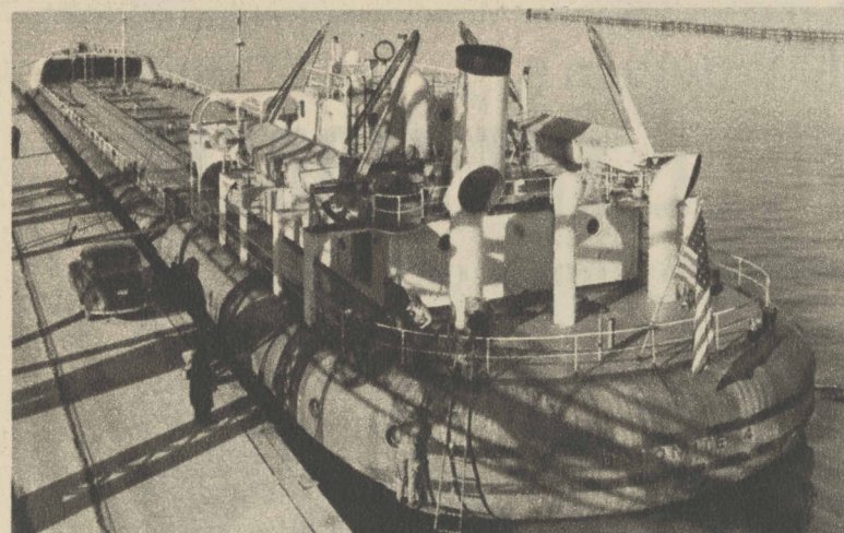
Dolomite-4, equipped for ocean service. It is unique in that its hold tanks are lined with pure nickel, hence noncorrosive.
