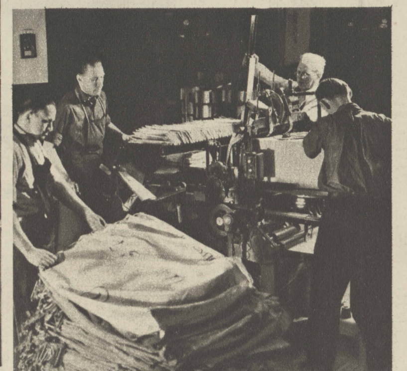
SPEEDS TRIBUNES TO READERS: One of the five multi-mailers on which Tribunes for individual subscribers are stamped, addressed and wrapped at the rate of three copies per second. More than 30,000 square feet of floor space in Tribune Tower are required to handle the distribution of the Tribune's circulation of more than 900,000 daily, and over 1,100,000 on Sunday.
