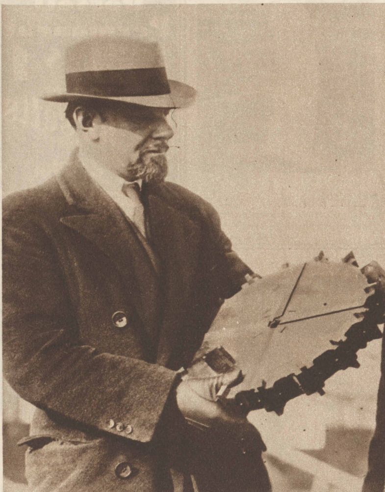
A DEVICE THAT MAY CUT A PATH TOWARD THE POLE —Sir George Hubert Wilkins, at Camden, N. J., inspects one of the circular ice saws to be used in his submarine cruise of the polar region. (Associated Press photo.)
