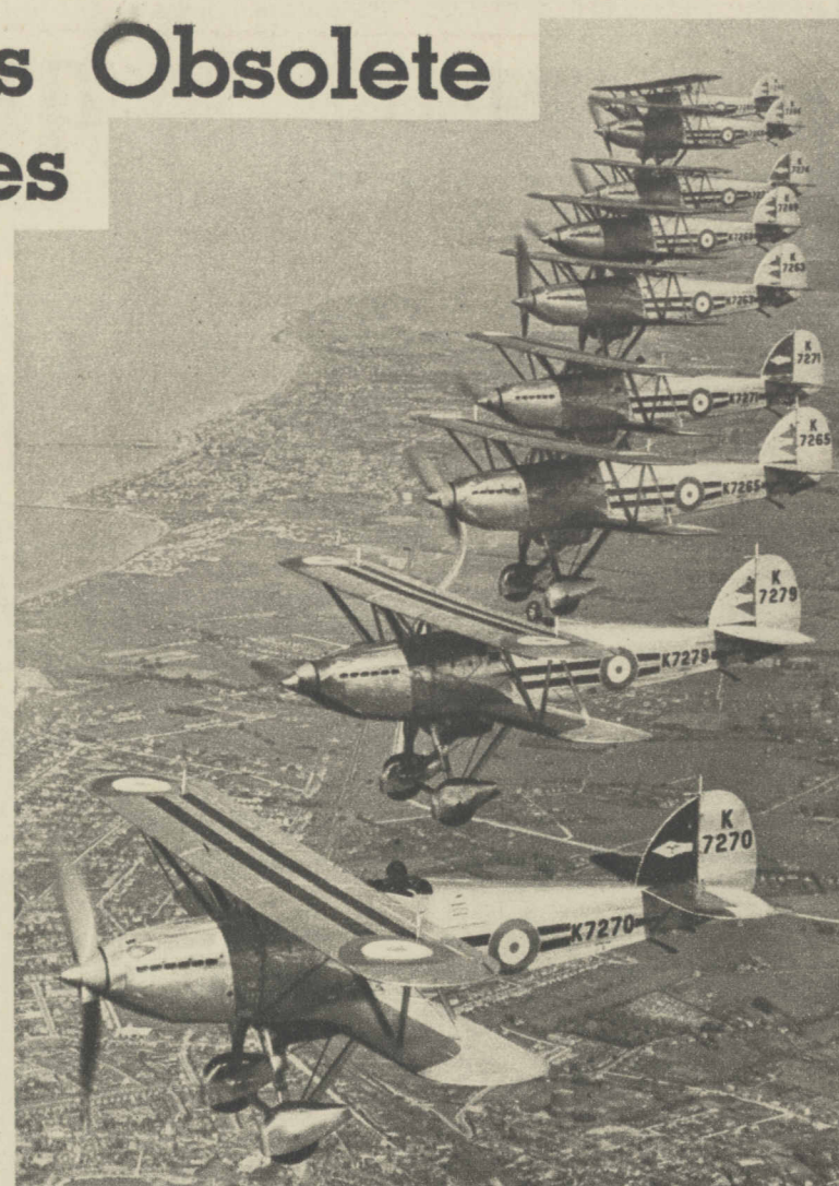
A squadron of British Hawker Fury war planes equipped with Rolls Royce Kestrel motors.
