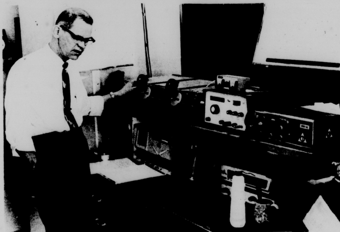
TORNADO WARNER--Harold Julien, chief weather meteorologist at Capital City Airport, will use this new system of communicating tornado warnings via seven radios. They are connected to ham operators, Civil Defense workers, State Police, area departments and other radio stations.
