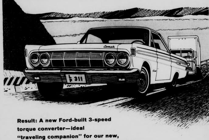
A completely new Ford Motor Company 3-speed automatic drive for 1964 delivers improved passing performance...smoother acceleration . . . better start-ups (up to 35% higher torque multiplication in Low) . . . more flexible downhill braking . . . quieter operation in Neutral.
