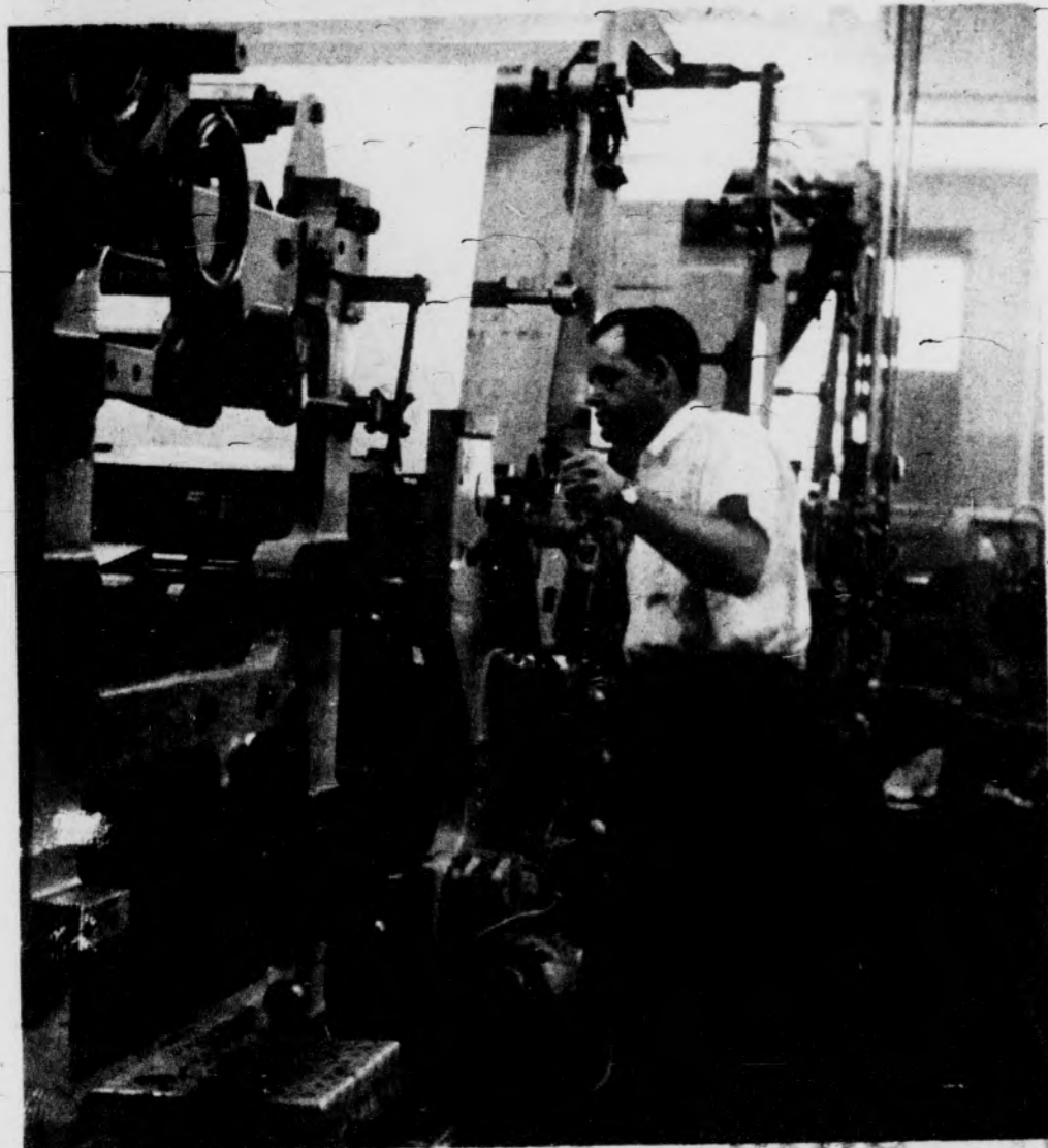
FINAL PRESS CHECK--Ready to start the press, Charles Webb sets the compressed air valves which will apply pressure to the printing surface.
