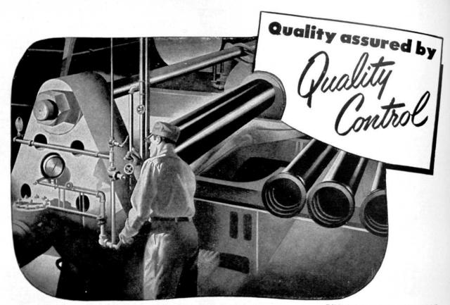
Nobody can buy a length of cast iron pipe unless it has passed the Hydrostatic Test at the foundry. Every full length of cast iron pipe is subjected to this test under water pressures considerably higher than rated working pressures. It must pass the test or go to the scrap pile.
