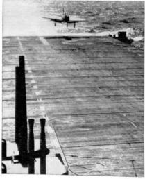
Landing at Sea. When a fighter pilot lands his plane on a flattop, one of his biggest problems is stopping the plane. To help him, a hook attached near the plane's tail engages one of the galvanized wire cables, mounted on spring brackets, that stretch across the deck. The resiliency of the cable, plus the bracket action, helps the plane to stop promptly and safely.
