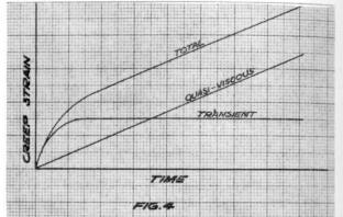
From Figure 3 it can be seen that the flow associated with the constant B or transient creep is more important at low stresses than at high. On the other hand, at high stresses the quasi viscous flow becomes the dominant one. Andrade has shown that the same is true for temperatures; transient creep is more important at low temperatures, quasi viscous creep at high temperatures.
