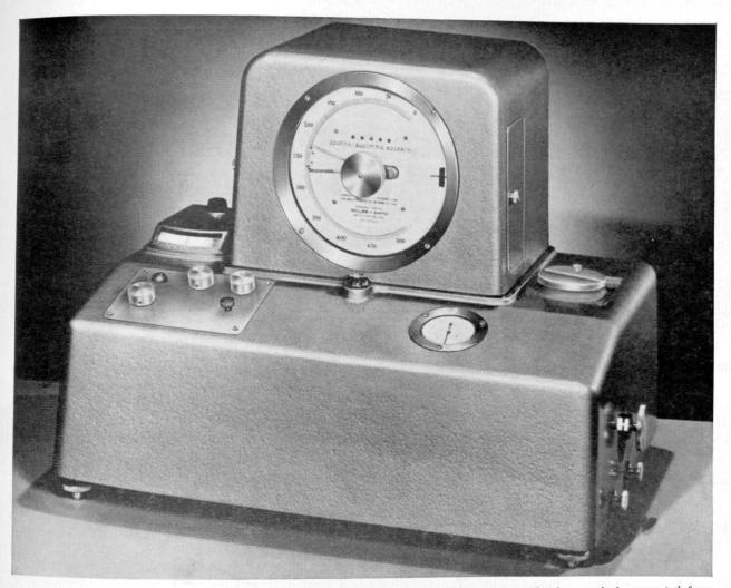
**THE PERCENTAGE** of hydrogen in liquid hydrocarbons can be determined by making two simultaneous measurements on the sample to give (1) density and (2) the absorption rate for beta rays. The weight percentage of hydrogen in the sample is computed from these measurements and a calibration curve. The new instrument shown here, a Standard Oil development, measures the beta ray absorption rate.
