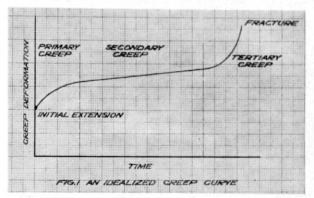
This also very well brings out the great dependence the creep deformation has on stress and temperature. At low stresses and low temperatures secondary creep
