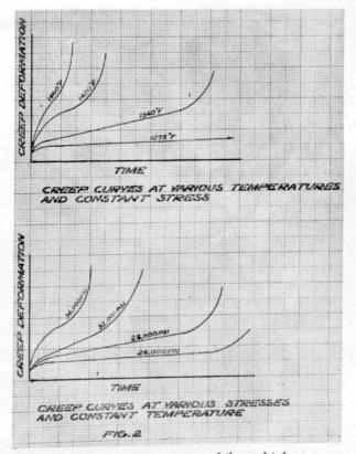
plays the most important part, while at high stresses and high temperatures the creep curve practically consists only of the primary and the tertiary stages.
