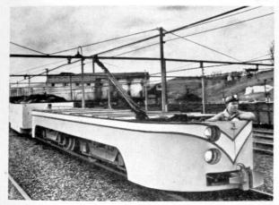
A modern high-speed, 30-ton mine locomotive hauls loaded coal cars from gathering tracks to coal tipple economically, quickly, and with a high degree of safety.
