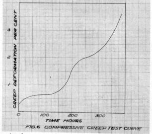
Another reason given for the tertiary creep stage is the metallurgical changes like overaging, recrystallization and phase changes in the specimen. Metallurgical transformations affect the creep characteristics very much, but in many tests no metallographic changes are seen, while the accelerated creep rate still occurs. Thus the precise mechanism of this last stage of creep is very obscure and much investigation is needed to explain it.
