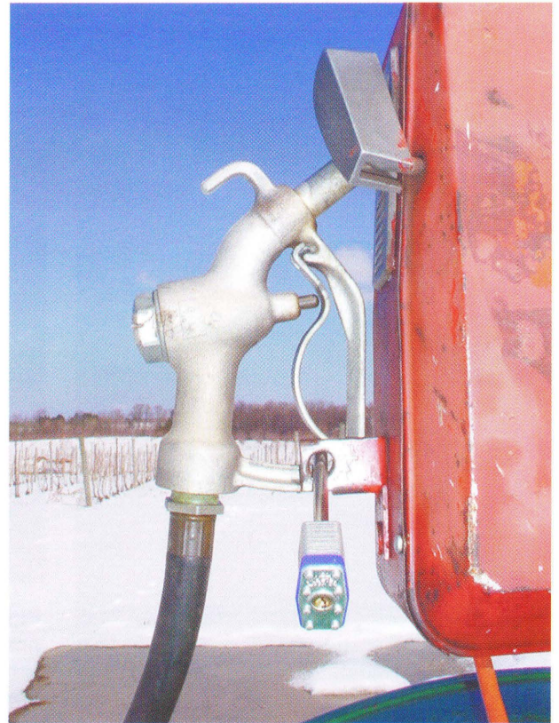
Fig. 8. Automatic shut-off nozzle, with lock to prevent unpermitted users from contaminating your farm or causing fire hazard.
