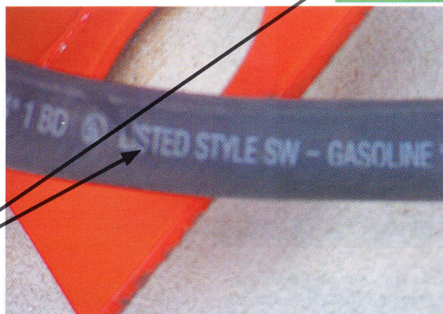
Fig. 10. Hose must be UL-listed/approved for the type of fuel.
