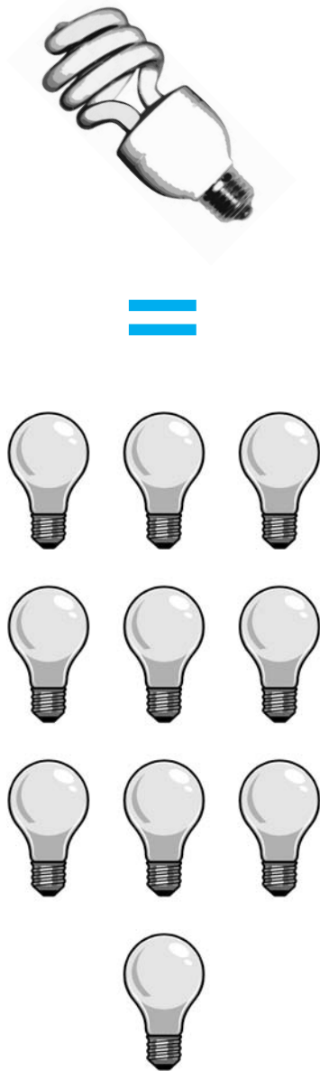
Figure 2: Light bulb comparison. Compact fluorescent bulbs—even though they cost more—last 10 times longer than ordinary bulbs. In the long run, they cost much less to operate.
