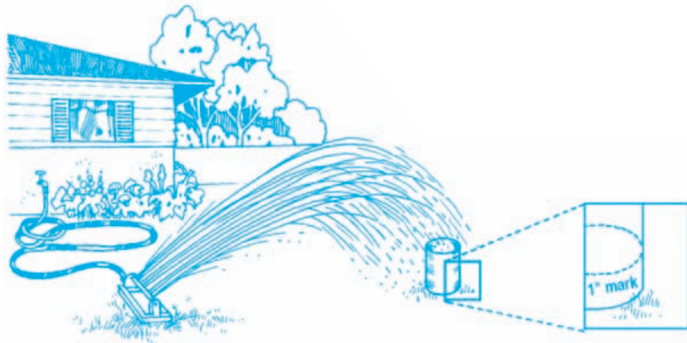
Figure 4: Sprinklers vary. To determine how much water your sprinkler is delivering, place a can with straight sides in the sprinkler path. Measure with a ruler the amount of water delivered in a given time period (example: 1 hour).
