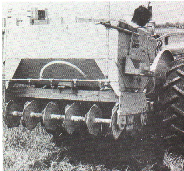
Fig. 4. The Zip Seeder, specially designed to seed legumes and grasses with fertilizer, has produced good stands in sods suppressed with paraquat.
