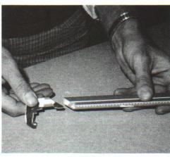
Step 4. Insert a corner brace into each end of one of the pieces and attach two more sides so you have a "U" shape.
