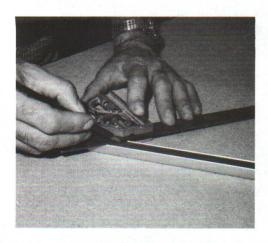
Step 1. Mark off a 45° angle near one end of the material.
