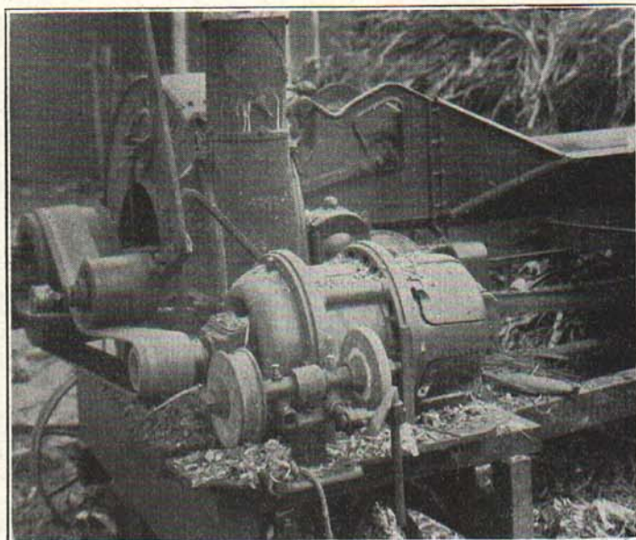
Five H. P. Electric Motor mounted on frame of cutter. Pulleys two feet apart at centers. Idler used on belt to give proper tension. Too tight a belt ruins the bearings of machinery.
