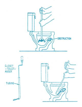
First try a "plumber's friend" or plunger. A plunger for the toilet is different than one for a lavatory, although there is a type which can be used for both. If this does not clear the stoppage use a plumber's snake made for a toilet. This differs from a lavatory snake because it has a section of tubing which can be pushed into the liquid in the toilet.
