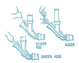
start the point of the tape down the drain. If the tape hits an obstacle, ram it back and forth until it clears. When it clears you will probably hear the water gurgle as the pipe empties. With a hose flush the drainpipe before replacing the plug.
