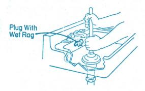
Next use a "plumber's friend" which applies first pressure and then suction to the plugged drain. To provide the suction and pressure, smear a good layer of petroleum jelly on the edge of the rubber stopper. Then plug the overflow with a wet rag so the air will not short circuit through the overflow pipe. Pump the plunger to loosen the stoppage. If this loosens the plug, rinse the drain with hot soapy water.
