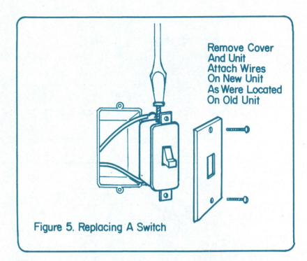
Wall Switch - When the light is out, first replace the bulb with one you know will light. With the new bulb in the socket turn on the switch. If light doesn't go on, check the fuse box in the basement. If fuses are all good the problem is probably the switch.
