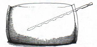
Fig. 2. Proper probing technique for bag sampling.
