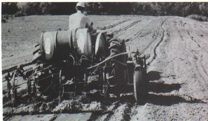
Figure 3. — A typical chisel type fumigant injector for use in pre-plant soil fumigation.
