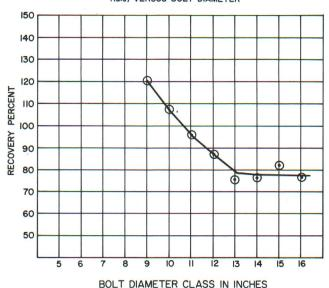
For bolt diameters from 13 through 16 in., recovery leveled off at approximately 78%. The average percent recovery for logs in this study was 86%. The waste occurred in the outside slabs, sawdust, and on a wedge-shaped center containing the pith.
