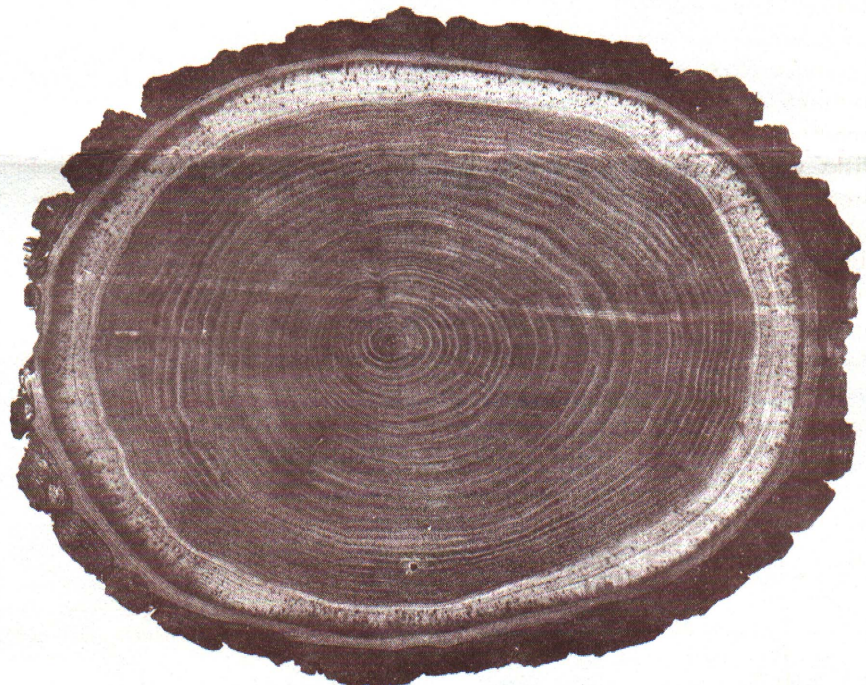
FIGURE 1. A Walnut cross section wood disk treated with Polyethylene Glycol (PEG) to prevent checks and cracks.
