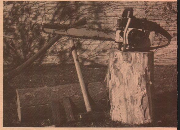
Figure 3. A minimum of tools is required to harvest your own wood. A chain say makes for faster cutting, however a crosscut or bow saw may also be used. All of these tools can be obtained from local hardware or farm supply stores.
