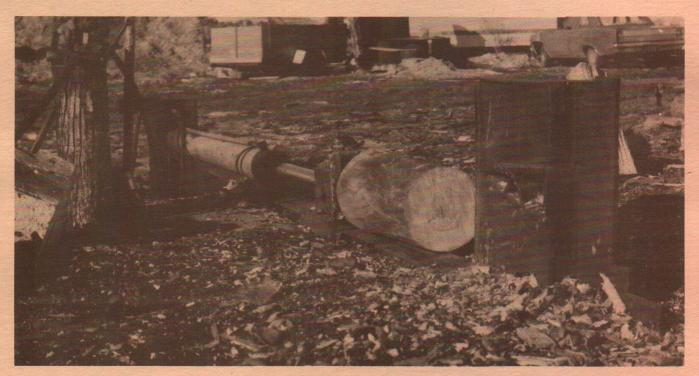
Figure 4. Where a large amount of wood is to be split, a power-operated splitting machine will reduce the amount of labor required while increasing the speed and ease of splitting. The hydraulic cylinder forces a block of wood against a stationary splitting wedge.
