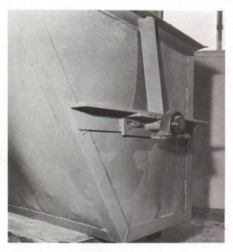
Fig. 1. Two methods of mounting bearings are illustrated in these pictures. Both are equally satisfactory. A  $3\frac{1}{2}$ " diameter hard rubber bottle stopper makes an ideal bumper. Rubber acts as a shock absorber and eliminates the noise caused by the tank dumping.
