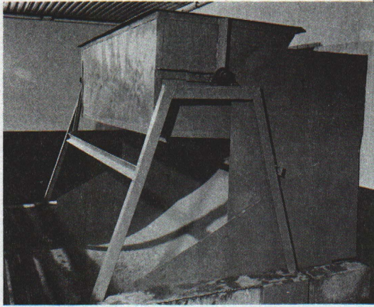
Fig. 2. Tanks can be mounted on a steel frame, poured concrete wall or a 6" concrete block wall. Likewise, the curved spillway can be constructed of concrete or metal. Use the material that fits your capabilities best.
