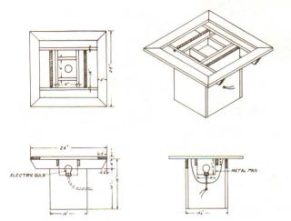
A simple plan for a water stand with light bulb to prevent water from freezing.
