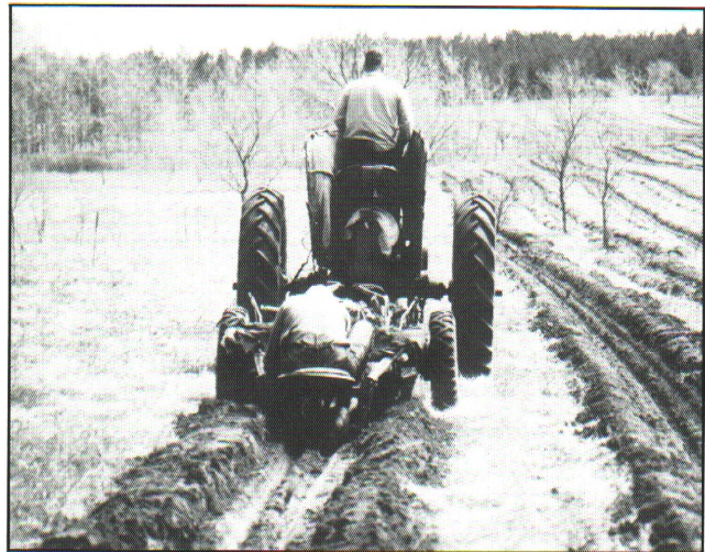
Figure 2: A scalper and furrowing disc.
