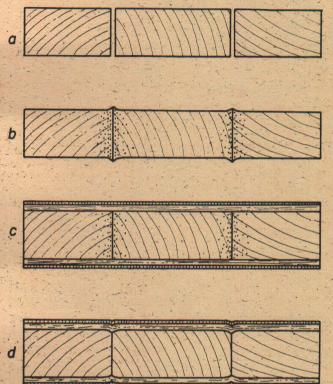
Figure 11. Development of sunken joints in lumber core panels. Dots indicate moisture absorbed from glue line.
