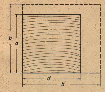
Figure 2. Swelling of square cross section when radial swelling is smaller than tangential swelling (a = a'; b - b'). Cross section remains rectangular but not square.
