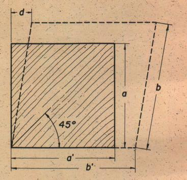
Figure 3. Swelling of square cross section when radial swelling is smaller than tangential swelling and annual rings oriented diagonally. (a = a'; b = b'). Values of "d" for square cross section with  $a = \frac{3}{4}$  inch: Silver Maple, 0.012 in.; Yellow Poplar, 0.009 in.; Yellow Birch, 0.006 in.
