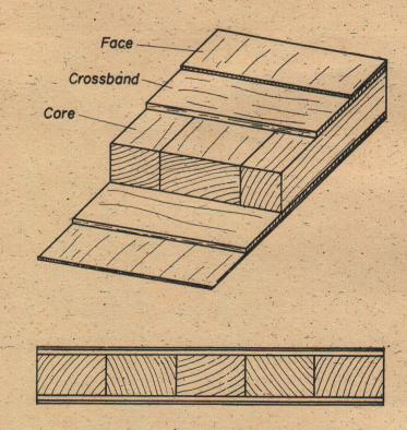
Figure 9. Construction of lumber core panel.
