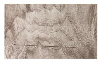
Figure 8-Rotary cut black walnut veneer. Note wide separation of growth ring ends in horizontal direction.
