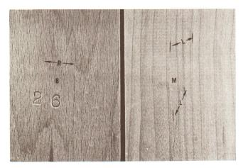
Figure 22—Beech, B, tangential surface with broad rays, R. Maple, M, with smaller rays not readily seen. The dark lines, L, are "mineral streak" a discoloration common in maple.
