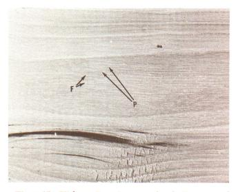
Figure 15—Hickory. Pores in narrow bands, P, separated by smooth hard surface, F.
