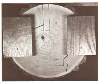
Figure 4—Cross-section of a log showing sapwood, S, heartwood, H, Quarter sawn board with radial surface, R, plain sawn board with tangential surface, T, and area from which they were cut.
