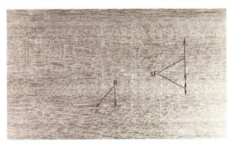
Figure 20 — Red Lauan. Radial surface with prominent rays, R. Stripe figure, SF, consisting of alternating bands of varying light reflection.
