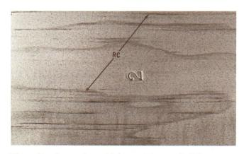
Figure 11 - Sugar pine with large resin canals, RC.
