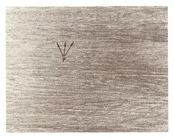
Figure 21 - Lauan with large pores, P.
