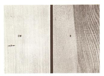
Figure 23—Cottonwood, CW, with barely visible pores, P. Yellow birch, B, showing contrast between heartwood and sapwood.
