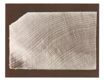
Figure 6—Cross section of sugar maple, a diffuse porous hardwood.
