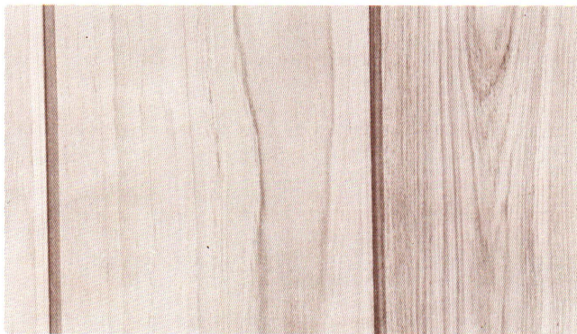
Figure 14—Tangential face of teak.
