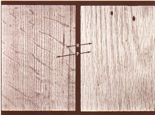
Figure 7—Red oak radial surface with prominent rays, R, on left, and tangential surface on right. Earlywood pores, P.
