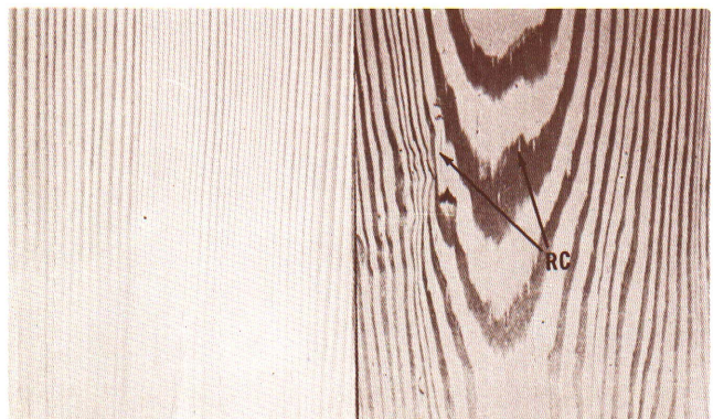
Figure 10—Radial surface of douglas fir on left, Tangential surface of southern pine on right showing resin canals, RC.
