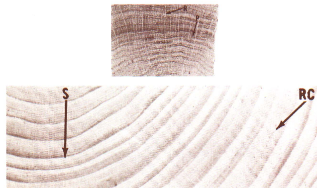
Figure 5—(Top) cross section of red oak, a hardwood with large pores, P; rays, R. (Bottom) southern pine, a softwood with dense latewood, S, and resin canals, RC (dark or light "spots.")
