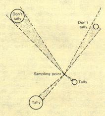
Fig. 1 How point sampling works in the field. Circles represent cross sections of trees at breast height, shaded areas indicate angle gauge projections from sampling point.
