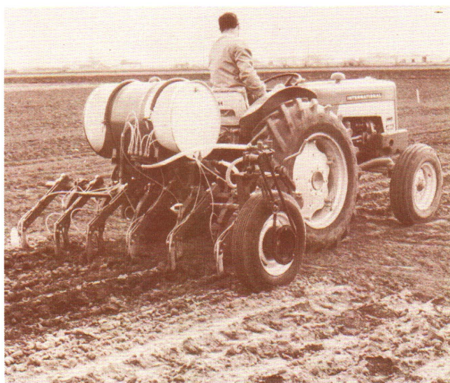
Fig. 12 — A pressure-type applicator using a wheel-driven pump for broadcast treatment.
