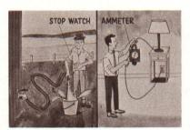
Suppose we fill a gallon pail with water from the garden hose while noticing how much time it takes to fill the pail. This would tell us the *rate of flow of water* through the hose in gallons per minute. Similarly, with an instrument called an *ammeter*, we can measure the *rate of flow of electricity* through a wire. The rate of flow of electricity through an electrical system is measured in *AMPERES*, or *AMPS*, for short.
