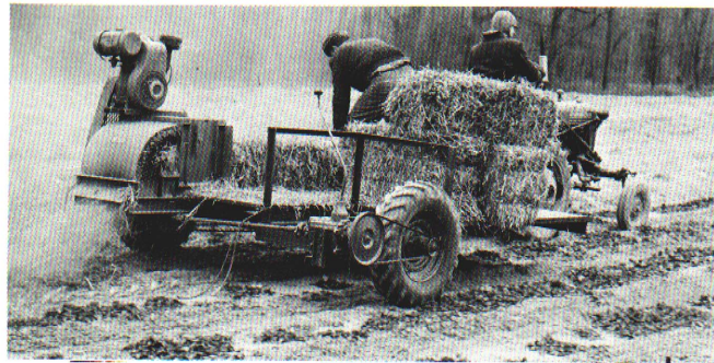
Fig. 15 – Specially constructed equipment readily deposits mulch over strawberry row. (Photo courtesy USDA Photo Service.)
