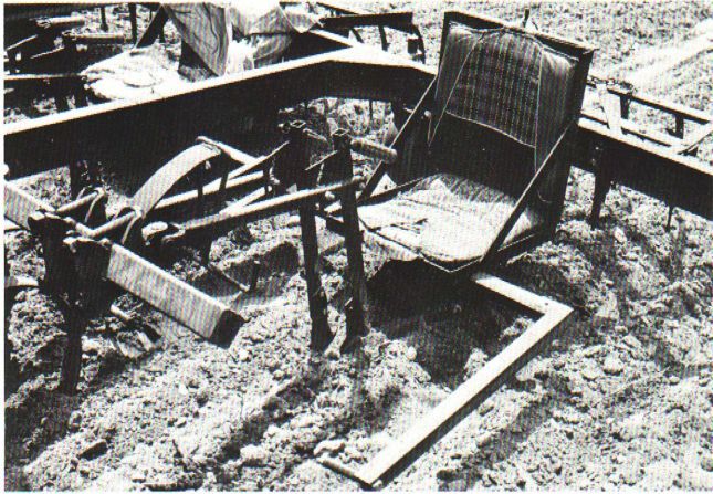
Fig. 8 - A 'wobble hoe' drawn behind a tractor-mounted cultivator. Rider moves (wiggles) cultivator shovels around strawberry plants to cultivate in the row between plants.
