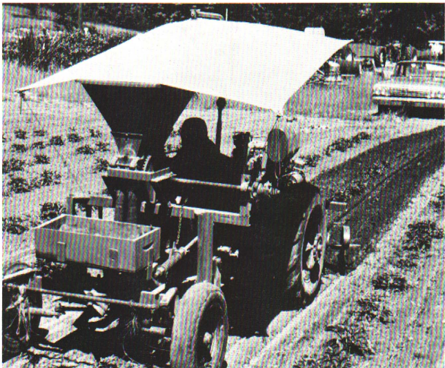
Fig. 9 - A type of power hoe used in some Michigan strawberry fields.
