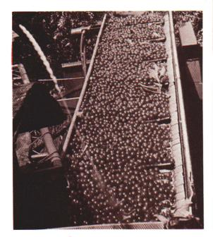
Fig. 7—An overloaded conveyor caused by an excessive harvesting rate. Overloading increases fruit damage, such as bruising and eventual scald.
