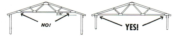
Figure 1 - Two types of roof trusses used in Michigan Farm Buildings (incorrect - left; correct - right).
