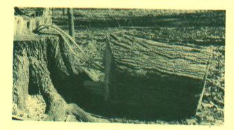
Figure 7 — Pulled-grain caused by an improper undercut and poor felling technique has resulted in the loss of many board feet of valuable hardwood.
