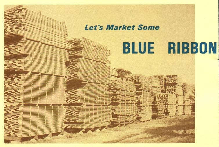
Figure 1 — Hardwood lumber from the Blue Ribbon species is highly prized by the furniture industry. Here, lumber is stacked for air-drying prior to being kiln-dried.
