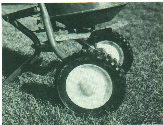
Centrifugal (broadcast) type fertilizer spreaders distribute materials rapidly with minimal overlapping.
