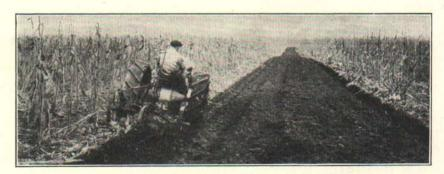
Fig. 3. Wide Bottoms Plow Whole Stalks Cleanly.
