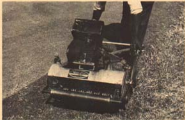
Figure 5. Applying peat-sand mix as a topdressing for a golf green. Top picture shows an aerator used for punching holes in golf green. Lower figure shows the spreading and raking of the soil mix into the holes with a steel mesh mat.
