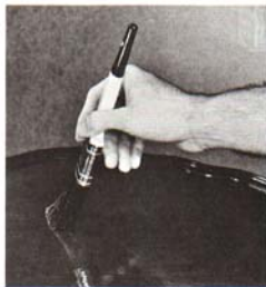
Hold brush as shown. Apply sealer, lacquer, varnish, and other transparent finishes with the tips of the bristles. Keep brush from clogging up.
