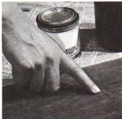
Filler is flattened and ready to wipe off if it rolls into a ball when you run your finger over the surface.
