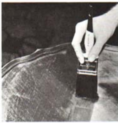
Apply stain with brush, cover thoroughly. Stain only one surface at a time such as leg, top, etc.
