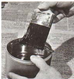
Straight stiff wire on coffee can makes a good container. Dip bristles to about one-third length and wipe off excess on the wire.
