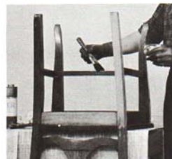
Start at the bottom first. Set chairs up-side down. Begin on underside of rungs.
