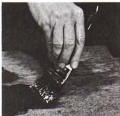
Brush thinned paste wood filler to cover an area not over 2 square feet in size.
