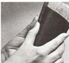
In sanding topcoats, use waterproof abrasive paper around a wood block with pad of felt or sponge rubber between paper and block.
