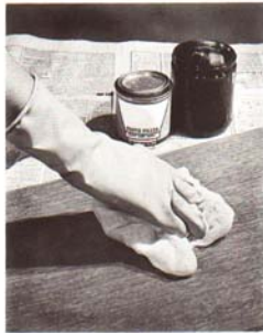
Finish wiping the filler, using cheese cloth with light strokes with the grain.
