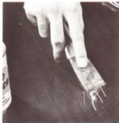
Tinted plastic wood applied with putty knife will repair deep chips and deep scratches.
