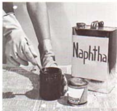
Stir paste wood filler to uniform consistency. Thin with naphtha or turpentine.
