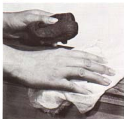
ing and wipe dry with a soft cloth. Then rub lightly with steel wool. As a final step, wipe surface clean to prevent iron rust from fine steel wool deposits.
