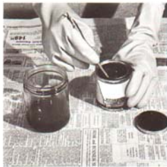
Mix pigmented stains thoroughly. Reduce color intensity with turpentine or paint thinner.
