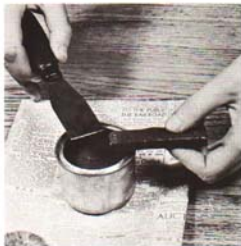
"Canned heat" can be used to melt a shellac stick for repairing deep scratches.
