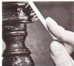
Stiff bristle tooth brush is handy in grooves or moldings to remove finish.
