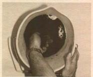
Mix the soil thoroughly—revolve the pail to ensure that a good mix is obtained.
