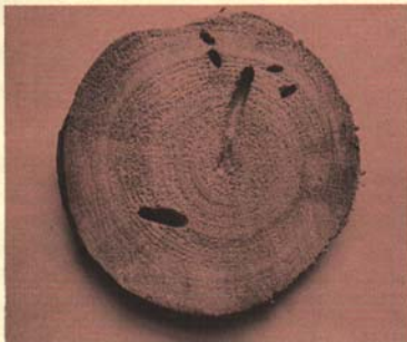
Feeding damage of buprestid (metallic wood-borer) larvae. The tunnels may be as much as \frac{1}{4} inch or more in diameter. The larval feeding damage of long-horned beetles is similar to the buprestids, but generally larger in diameter and less oval.
