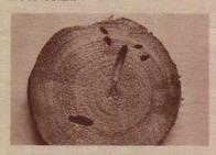
Feeding damage of buprestid (metallic wood-borer) larvae. The tunnels may be as much as ¼ inch or more in diameter. The larval feeding damage of long-horned beetles is similar to the buprestids, but generally larger in diameter and less oval.
