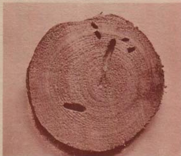
Feeding damage of buprestid (metallic wood-borer) larvae. The tunnels may be as much as \frac{1}{4} inch or more in diameter. The larval feeding damage of long-horned beetles is similar to the buprestids, but generally larger in diameter and less oval.
