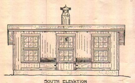
Fig. 3.—South Elevation—Sun light and ventilation are essential. This window and ventilator arrangement provides both.
