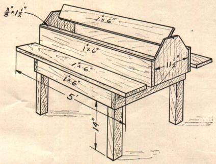
Fig. 13.—A simply constructed dry mash feeder. The revolving board on top prevents contamination of the feed.
