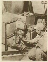
The hopper-bottom metal bin in foreground, coupled with the variable speed drive unit and changeable size augers in the bin, allow a wide range for metering grain, ground feed, and supplement. The rectangular metal bin (center) with a moving apron as a floor and the hoppered bin serve as meters or flow regulators for silage and cornage.
