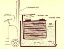
Fig. 1. Equipment of this type has been successfully used for the bulk disping of apples in scald-inhibitor solution. An adjustable box cover attached to the lift would simplify the operation nonvechat. Also, a motor-driven agitator should be employed to prevent settling of the active ingredient to the bottom of the tank.
