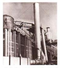
Fig. 30. The second step in converting wet wood waste into fuel briquets involves drying the previously hammermilled refuse in flash driers. The first stage of a two-stage dryer is shown here. See Item 19 in Fig. 27 for the location of this tower. (Photo: Summer Iron Works, a division of The Black Classon Company).
