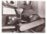
Fig. 29. As an initial step in the manufacture of briquets, this hammermill receives the hogged refuses from the sawmill and reduces it to a standard small size before drying in flash driers. The location of this equipment in the briquet plant is shown by Item 9 in Fig. 27. (Photo: Sumner Iron Works, a division of The Black Clawson Company).
