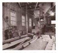
Fig. 31. Extrusion through this press is the final major step in the manufacture of fireplace-size log briquets from wood waste. Dry refuse (of controlled particle size) is admitted from the overhead storage hopper. The log tube extends to the left. Capacity of this machine ranges up to 2 tons per hour. See Item 37 in Fig. 27 for the location of this equipment in the manufacturing process. (Photo: Summer Iron Works, a division of The Black Clawson Company).
