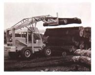
Fig. 11. All movement of logs in the mill area (from log sorter to log storage and from log storage to sawnill deck) is handled by this versatile four-wheel drive fork lift. It is estimated that one operater with such a machine can keep the mill supplied with 40,000 board-feet of logs per shift. (Photo: Pettbone Mulliken Corp.)
