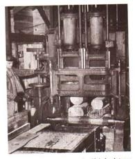
Fig. 17. Sash gangsaw measuring 32 inches between styles or sash, with a stroke of 13 inches, depth of cut of 14 inches, and with 13%-inch maximum opening between feed rolls and press rolls. Note individual pressure cylinders actuating the split press rolls to permit feeding of multiple cants. By feeding cants in multiples, the gangsaw can maintain a production of 40,000 board-feet per 8-hour shift. (Photo: Wickes Brothers Division, The Wickes Corp.)
