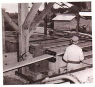
Fig. 20. The "Electric Swede" is equipped with smooth rolls and a 3-horsepower motor. In this operation, the grader pulls lumber to be resson a few inches out from the lumber line where it is caught by the rolls of the "Electric Swede" and jerked onto a transfer chlas leading to the resaw. (Photo: Moore Dry Kiln Co.)
