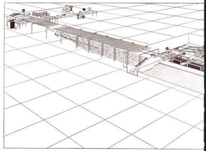
Fig. 12. Layout of sawmill<sup>\*</sup>. The sawmill is designed to utilize logs at an average rate of one every 18 seconds, or 40,000 board-feet per 8-hour shift. The logs average 9 inches in diameter and 10 feet in length. Pages 13 through 19 of the text describe the flow of material through this portion of the manufacturing process.
