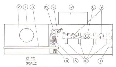
Fig. 28. Briquet plant layout (four machines).\* Each of the four machines in this particular layout has a capacity of a half ton per hour. The plant is designed to operate around the clock for 50 weeks out of the year and, thus, has a capacity in excess of the required 14,530 tons per year. The end product is wood briquets for fireplace use. "Source: Wood Briquettes Inc., Lewiston, Idaho.
