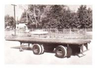
Fig. 8. Twenty-ton capacity trailer with 109-inch tandem to permit maximum loading and still meet local load limitations. Because of the necessity of hauling numerous short logs that develop along with the tree-length logs, a modified platform trailer may serve better than a conventional log trailer. Three such trailers, modified for carrying logs of mixed length, are required for the operation. (Photo: Trailmobile, Inc.)
