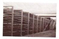
Fig. 23. View of a multideck lumber sorter looking from the sawmill in the direction of lumber movement and toward the lumber stacking station at the far end. Each level of lumber represents a separate sort. As each level fills with lumber, it is emptied onto powered chains that convey the entire sheet of stored boards to a mechanical stacker. (Photo: The Ivory Fine Co.)
