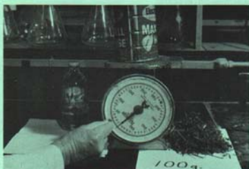
STEP #2 — Weigh container, with vegetable oil inside and screen. Set movable dial to "0".
