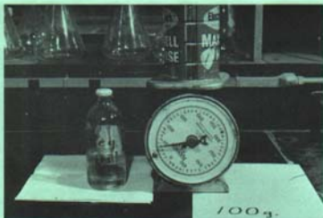
STEP #4 — After heating, set container and contents (oil, forage, screen) on scale. If dial was set at "0" in step 2, you are reading the dry matter "contained in 100 grams of forage or percent of dry matter".
